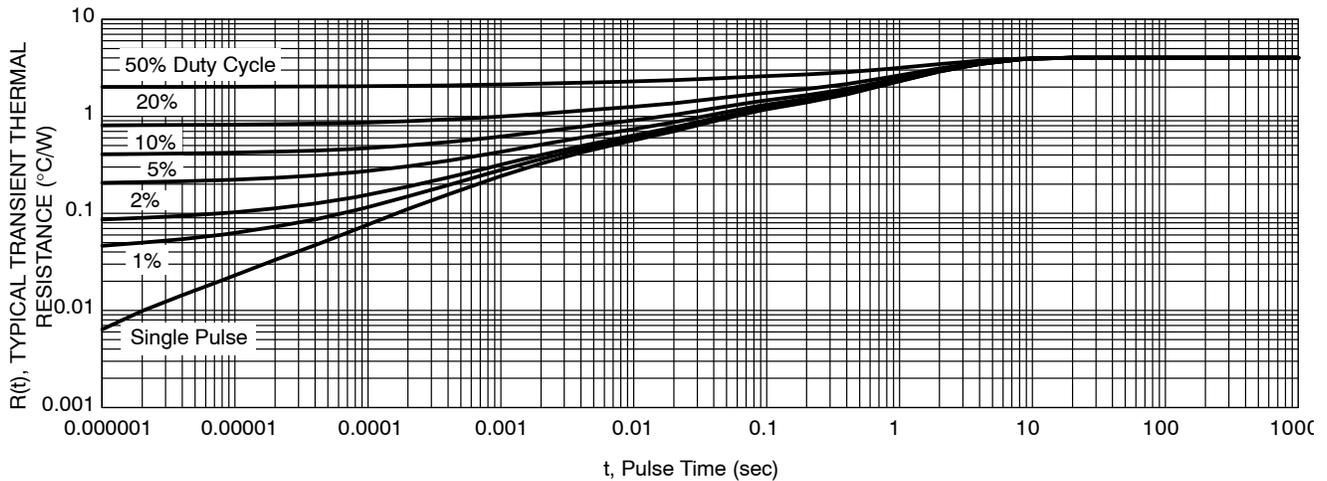
**Figure 8. Typical Transient Thermal Response for NTSJ30120CTG**
