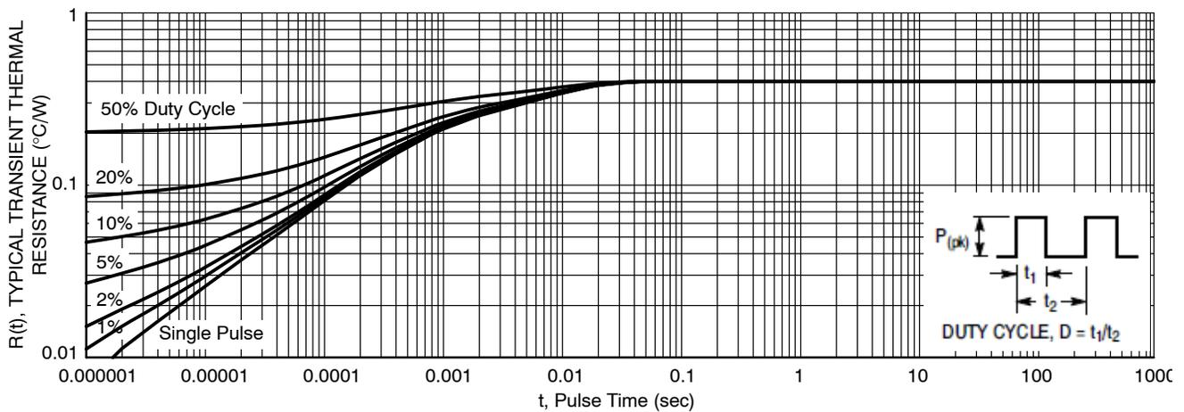
**Figure 9. Typical Transient Thermal Response for NTSB30120CTG**
