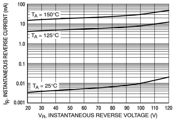
**Figure 2. Typical Reverse Current Characteristics**
